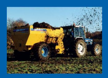
Machine capacity has grown from 5,910 litres to 14,500
