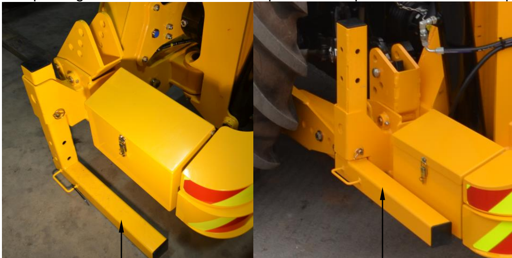
Parking stands in fully down position required when machine is being parked
