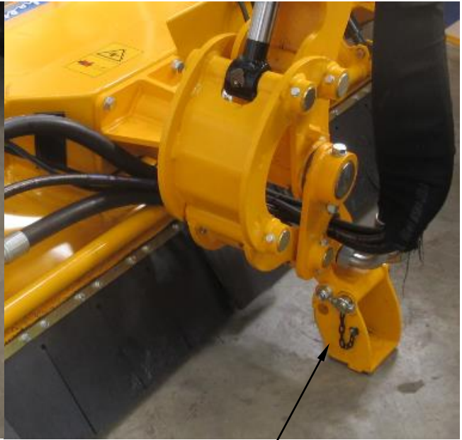
Pivot shoe foot fully down supporting cutting head
