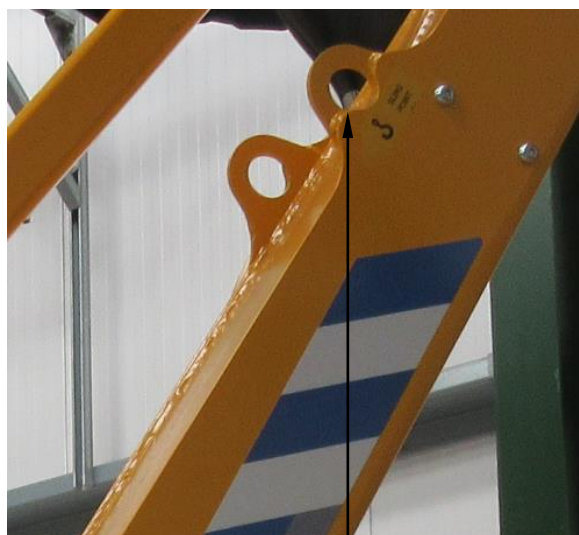
Sling point on inner boom.
