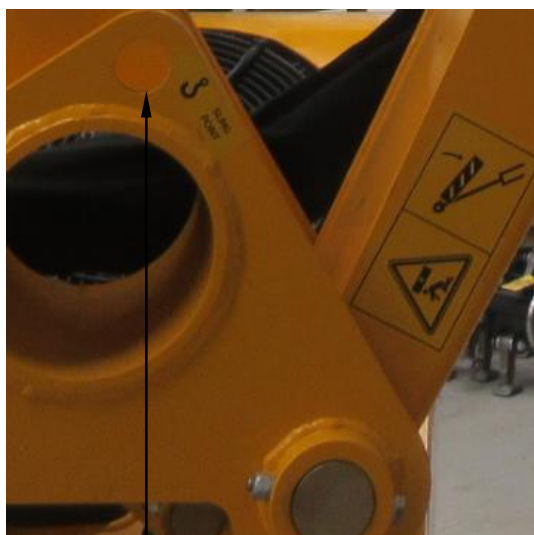
Sling point on main pivot rocker.
