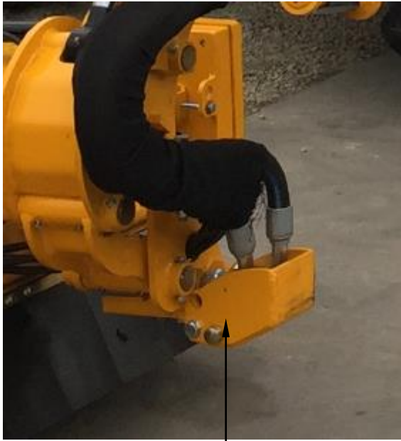
Pivot shoe foot fully up position
