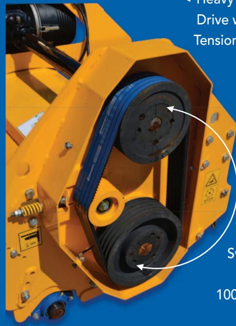
◀ Heavy Duty 5 Belt Drive with Sprung Tensioning System
